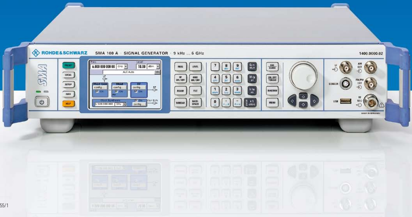
FIG 1 The analog R&S®SMA100A signal generator generates spectrally purest signals up to 6 GHz. Equipped with a new option, it also generates high-precision VOR/ILS signals for tests on air navigation receivers.
