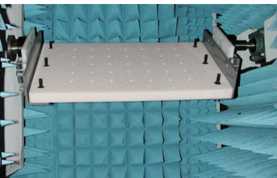
FIG 3 With the aid of manipulators made of low permittivity materials, the EUT can be rotated around all axes.
